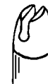
Replace the hazu . Use a rattail file to make a keyhole-shaped slot.
