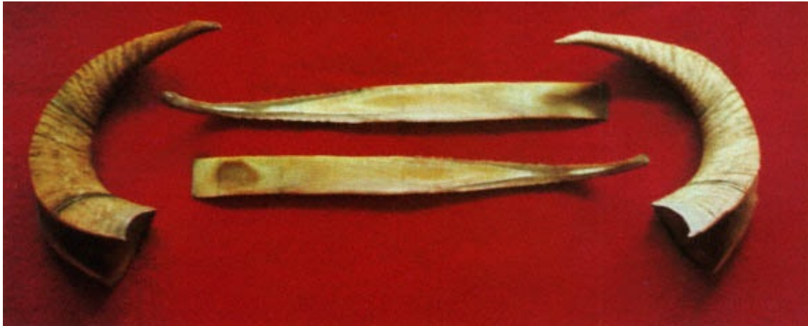
Two mountain-sheep horns after sawing off strips for bow limbs; and the two bow limbs after boiling, straightening, and rough shaping.
